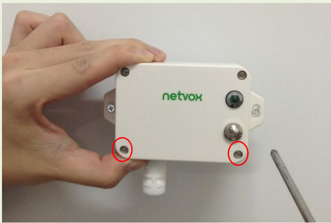
Screw hole diameter: Ø4mm
